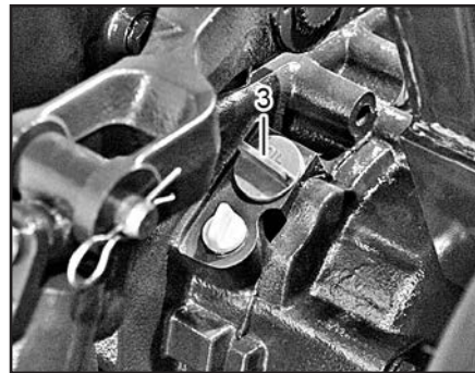
(1) Rear axle case (2) Transmission case (3) Oil Inlet
