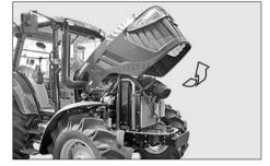
Lift the hood with hands slightly. Then, the hood is automatically opened by its damper.
