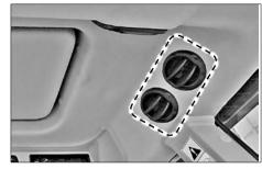
When using the A/C or heater in the fresh air mode, fresh air is drawn into the cabin through the filters installed on the left and right sides of the roof.
