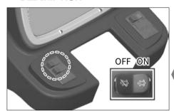
When the Forced DeSOx switch is set in the neutral position, the DeSOx operation is automatically performed for every 200 hours.
