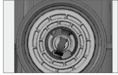
5. When no further rotation possible (after ca. 45°), then pull out the filter.
