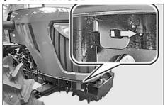
Push the hood opening handle under the hood front grill to the left as shown in the figure to unlock the hood.
