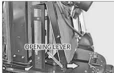
Turn the opening lever to access to the condenser and oil cooler.
