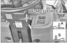
Press the hazard flasher switch in emergency to warn other vehicles in order to prevent an accident. The hazard flasher is operated regardless of the position of the main switch. Also, the turn signal lamp function is disabled while the hazard flasher is activated.
