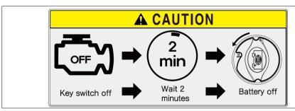
Turn the knob to "OFF" to disconnect the battery and back to "ON" to resume normal operation.
