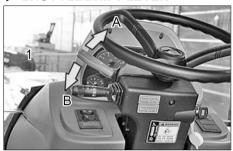
This device is used to select the driving direction between the forward and reverse directions.
