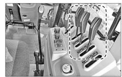
When using an attachment for an implement (rotavator, hydraulic plow, etc.), connect its hose to the proper port among the port A, B and C according to its use.
