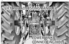
Turn the handle clockwise to extend the rod and turn it counterclockwise to retract the rod.
