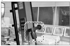
Hold the handle and push it outward to open the window.
