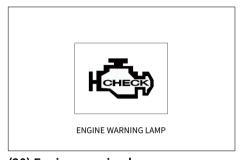
(20) Engine warning lamp It comes on when the engine is malfunctioning.
