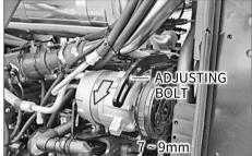
Check and adjust the tension of the A/C compressor belt regularly.
