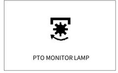
PTO monitor lamp indicates the state of the PTO shaft.
