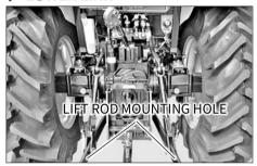
An implement can be attached to this. The installation type is Category II. (Implement mounting hole diameter: 25.4 mm)
