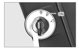
When key switch is in 「ON」 position, engine is automatically preheated as necessary.
