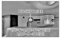
This lever is used to select the PTO speed.
